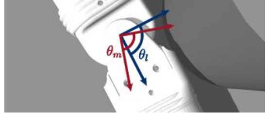
(b) A zoomed view of one of the joint module while colliding with obstacles. The motor position \theta_m is allowed movement through passive-compliance despite of the load position \theta_l being blocked by external obstacles.
