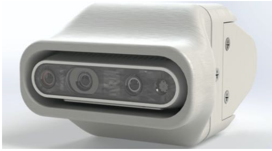
(a) The head module of Serpens with the Intel RealSense D435 stereoscopic camera.
