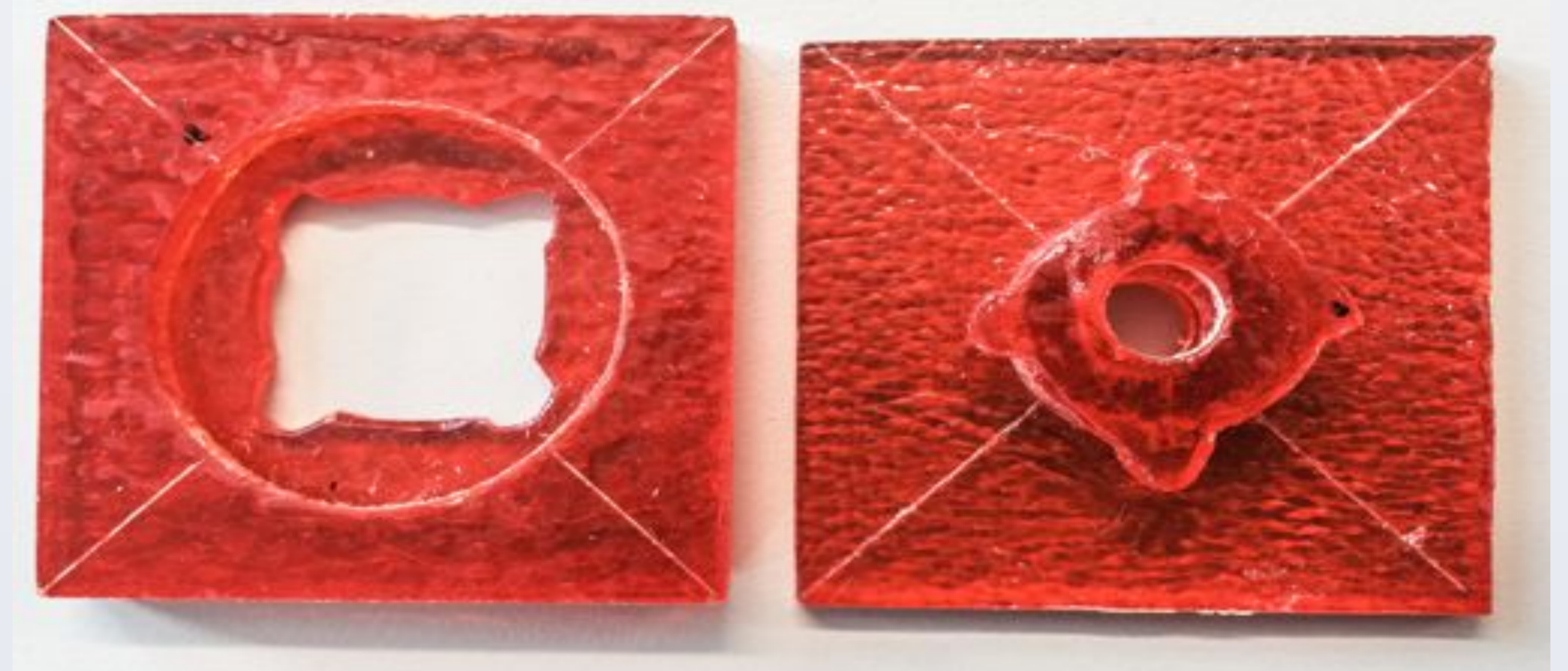
Fig. 2 The new self-locking concept mechanism allows for connecting the modules in a much more reliable way. Specially designed electrical contacts are embedded in the new self-locking mechanism allowing for easily powering each module.
