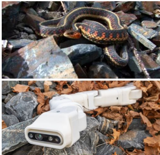
Fig. 1: A real snake locomoting in a cluttered environment (top); Serpens , the proposed low-cost ROS-based snake robot with series elastic actuator (SEA), precision torque control and a screw-less assembly mechanism (bottom).
