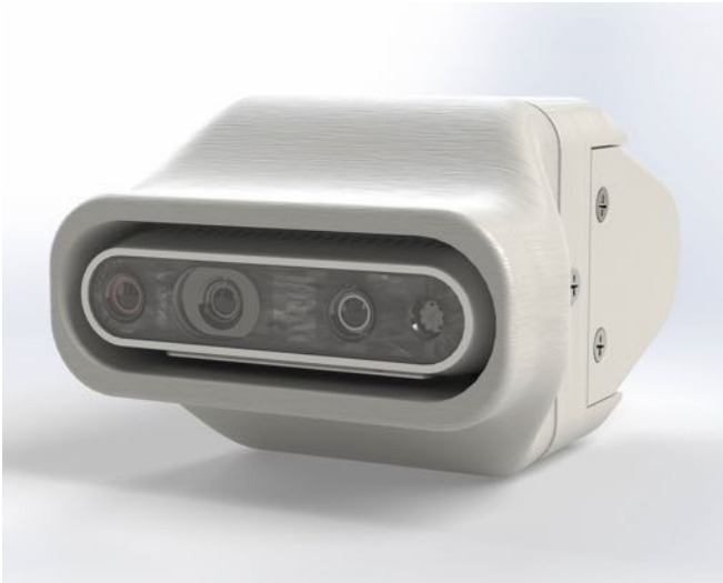
(a) The head module of Serpens with the Intel RealSense D435 stereoscopic camera.
