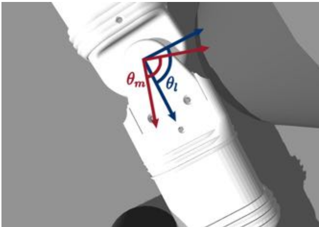
(b) A zoomed view of one of the joint module while colliding with obstacles. The motor position \theta_m is allowed movement through passive-compliance despite of the load position \theta_l being blocked by external obstacles.
