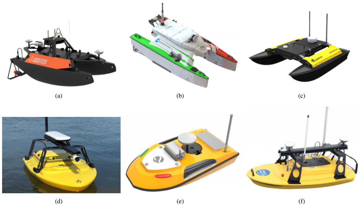
Fig. 2: Small size USVs with no more than 2 m length: (a) Otter, (b) SR-Surveyor M1.8, (c) Heron, (d) GeoSwath 4R, (e) SL20, (f) Z-Boat 1800 RP.
