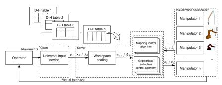
The proposed architecture provides the possibility of controlling the arms in position mode or velocity mode
