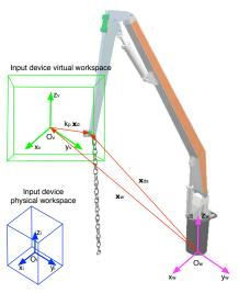
The proposed architecture allows for expanding and shifting the small-scale physical workspace of the input device to a virtual expanded workspace allowing the robot arm for more accurate and precise movements.
