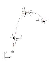
The torque  $\tau$  makes the snake straighten. This produces a counter force,  $f_{\tau}$ , acting at the obstacle  $o_3$ .
