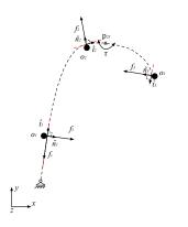
$\tau$  can be uniquely computed at any point. Given any point, s, on the path, it is possible to uniquely express the bending torque as a function of  $f_s$ ,  $f_1$ ,  $f_2$ ,  $f_3$ :
