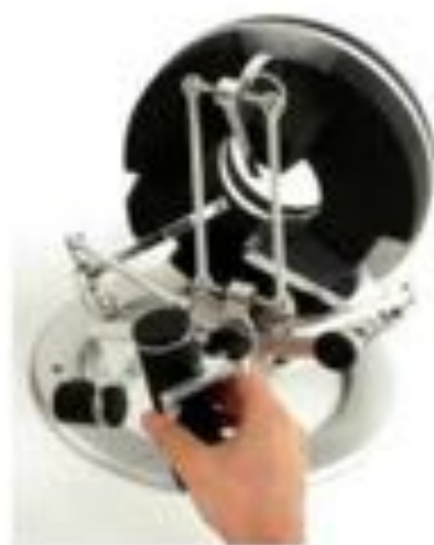
Fig. 5. The omega.7 haptic device from Force Dimension that was used as an input device.
