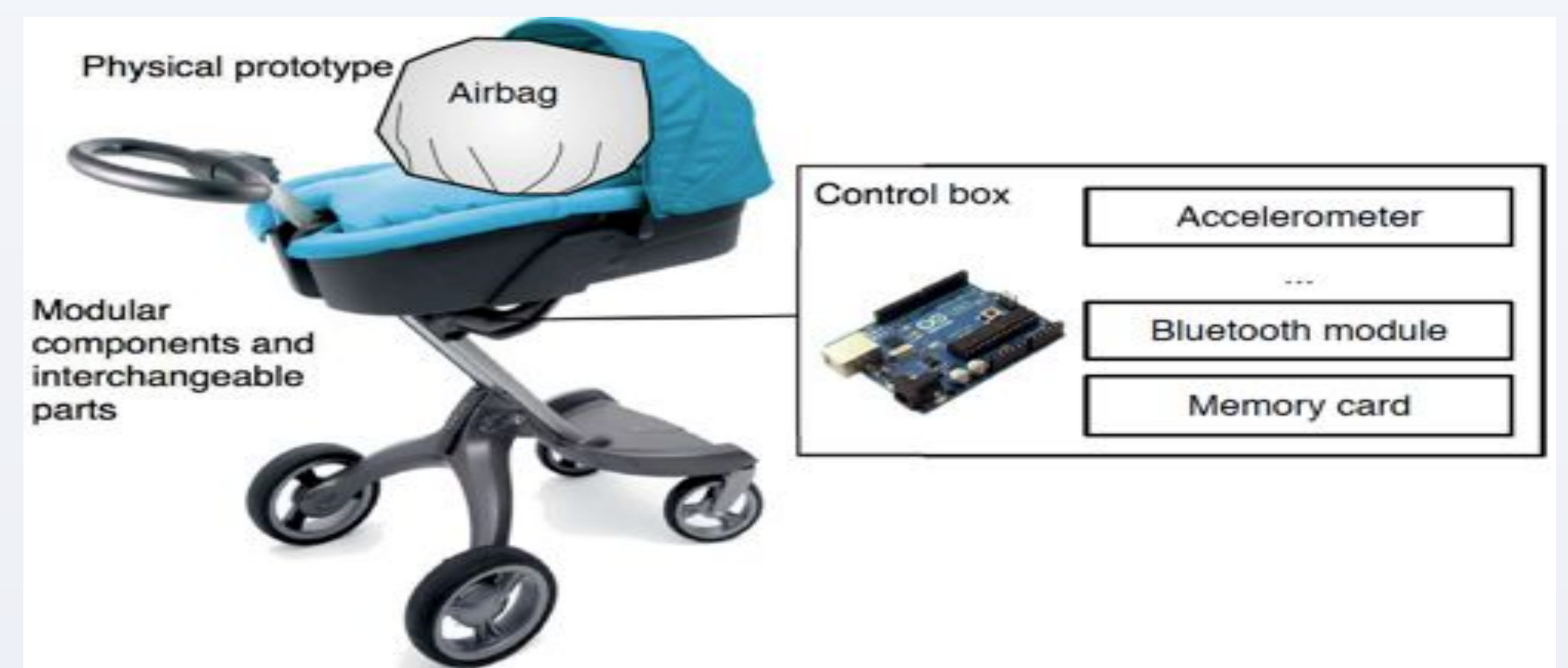
Fig. 3 Safety devices like airbags can be triggered on run-time.
