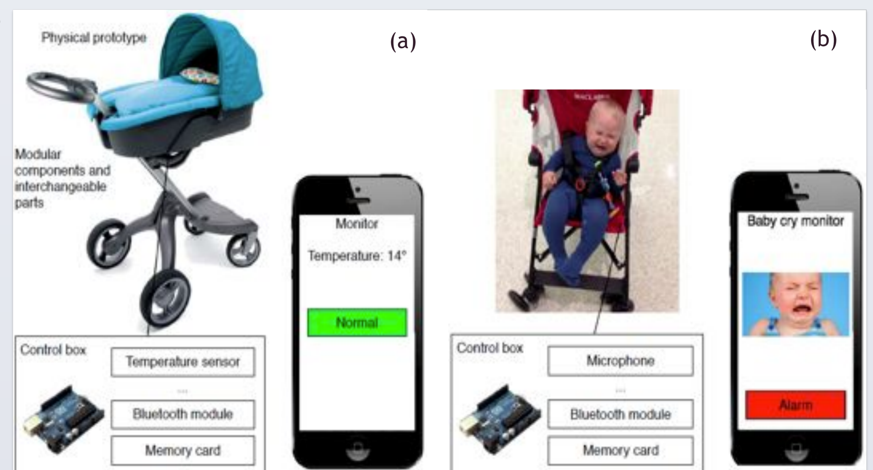
Fig. 4 The temperature and the sound can be monitored and transmitted to a mobile application.
